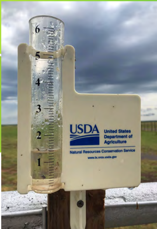
Rain gauges help to prevent overwatering.
