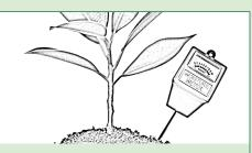
**MOISTURE** meters use the principle of electrical resistance to measure soil conductivity. Readings help determine proper watering.
